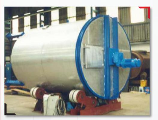
AISI 304 SS, Ø2200 - 4000, with Agitator and Ex-Proof Motor, Weight: 2500 kg
