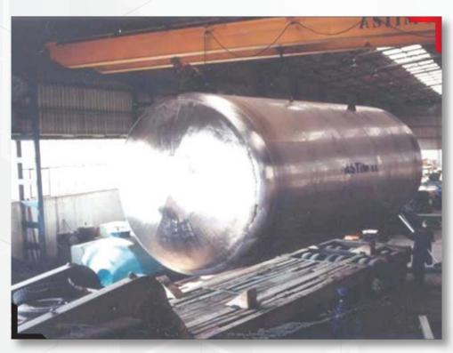
Ø4 m Diameter x 9 m Length, AISI 316 SS Material, Empty Weight: 9 Tons/Each
