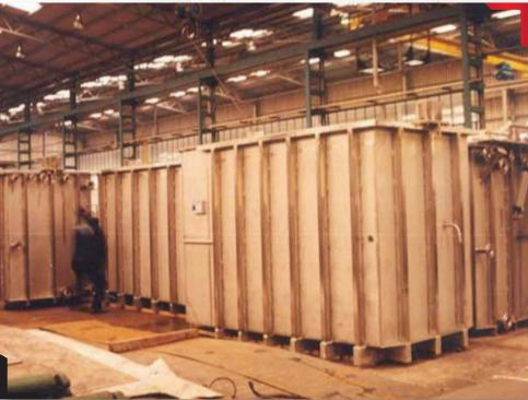
AISI 316Ti SS, Cover with Pneumatic Piston, Empty Weight: 2200 Kg/Each
