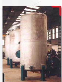
AISI 304 SS, Working Pressure 8 atu, Test Pressure 12 atu, Between Ø1600 - 2000 mm Diameters, Radiographic Controlled.
