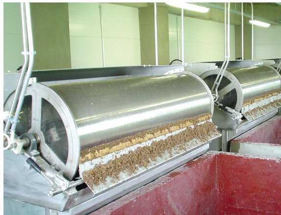
Series of Drum Screens used in brewery industry
