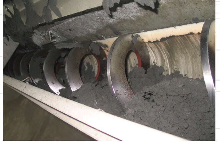
Shaftless Screw Conveyor used for sludge conveying
