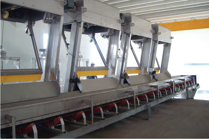
Belt Conveyor used to transport screenings
