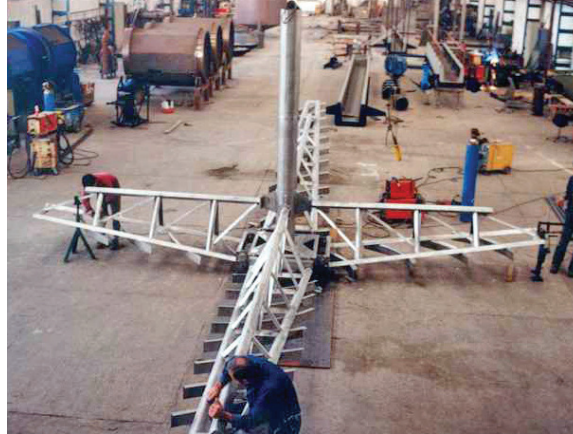
Central Driven Grit Scraper
