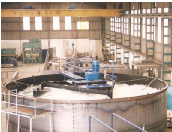
Vertical Shaft Turbine Aerators during efficiency test
