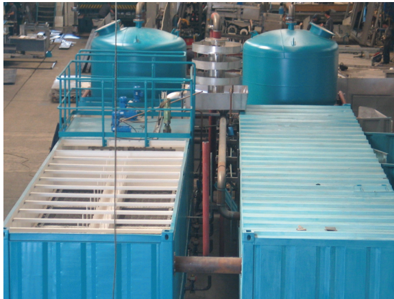
80 m 3 /h capacity CPWTP pre-assembled in factory
