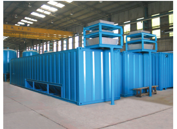
2 x 80 m 3 /h capacity CPWTP during pre-assembly
